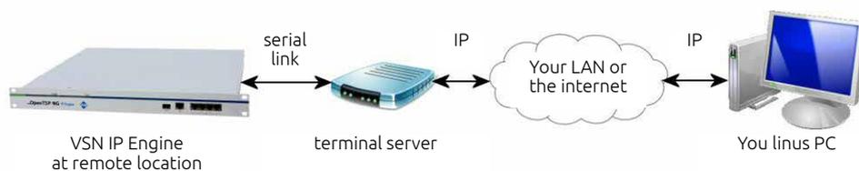
**Figure 2: Using a terminal server for debugging**
